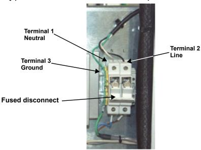
The AC wire should be pulled from the left (top access recommended) and through the rear top access panel (see **Figure 33**). Run the AC wire along the underside of the top cabinet frame rail from the rear to the front of the cabinet. Terminate the AC wire at the fused disconnect (pictured in **Figure 32**; see also **Figure 26**).
